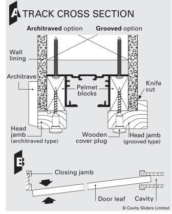
2 Remove door from track (drawing B, C, D). Fit the club end of the adjusting spanner over the hexagonal nut at the bottom of the hanger pin (drawing C).
